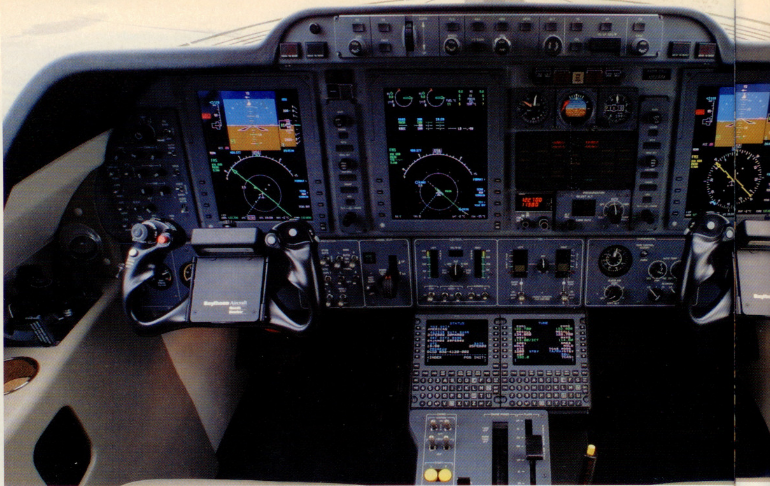
Collins' Pro Line 21 avionics adorn the Premier I's front office. Master them, and you've mastered the airplane.
